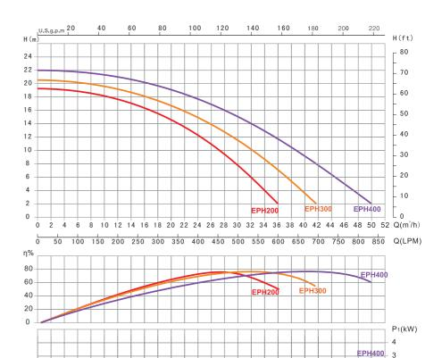
Remarks: Flow curve information based on 220V/50Hz motor.
